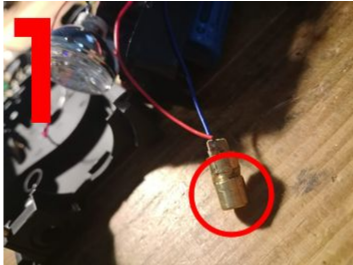
Adjustment and gluing of the laser lens
